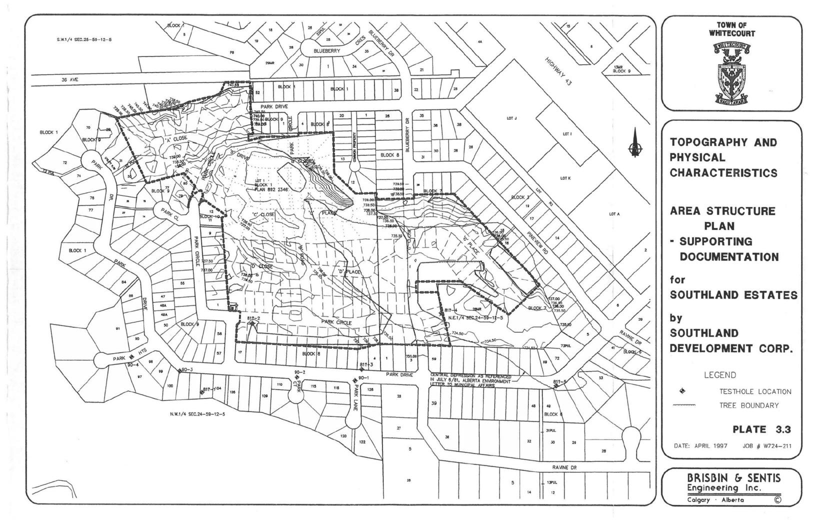
Park Drive (*south leg*) showed 3± m of sand over a silt layer. These test pits were dry. Prior to final design, a geotechnical investigation consisting of some ten test holes will be undertaken. This is currently scheduled for April, 1997.
